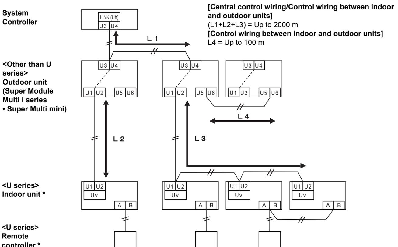
\* The wiring specifications in the system diagram above are the same even when the indoor unit or remote controller are other than the U series.
