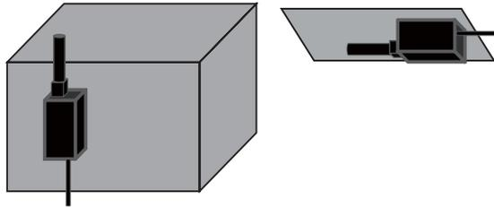
\* Install so that the power cable that connects to 220-240 V AC does not face upward.
