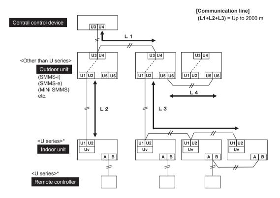
\* Even if the indoor unit and the remote controller are "other than U series", the wiring specification are the same.
