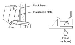
For detaching the indoor unit from the installation plate, pull the indoor unit toward you while pushing its bottom up at the specified parts.
