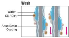
Reduces water and oil formation and prevents dust from sticking to the unit coil.
